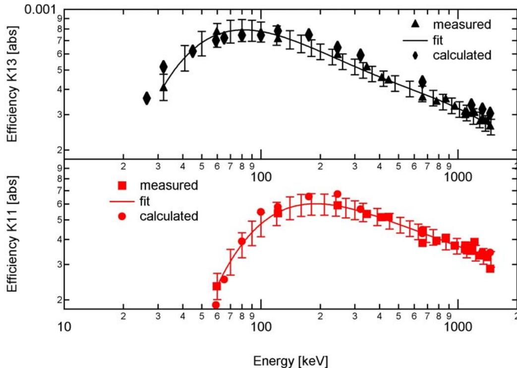
Figure 3.1. Efficiency curves for the p-type HPGc (K11, lower) and n-type GAMMA-X HPGc (K13, upper) detectors.
