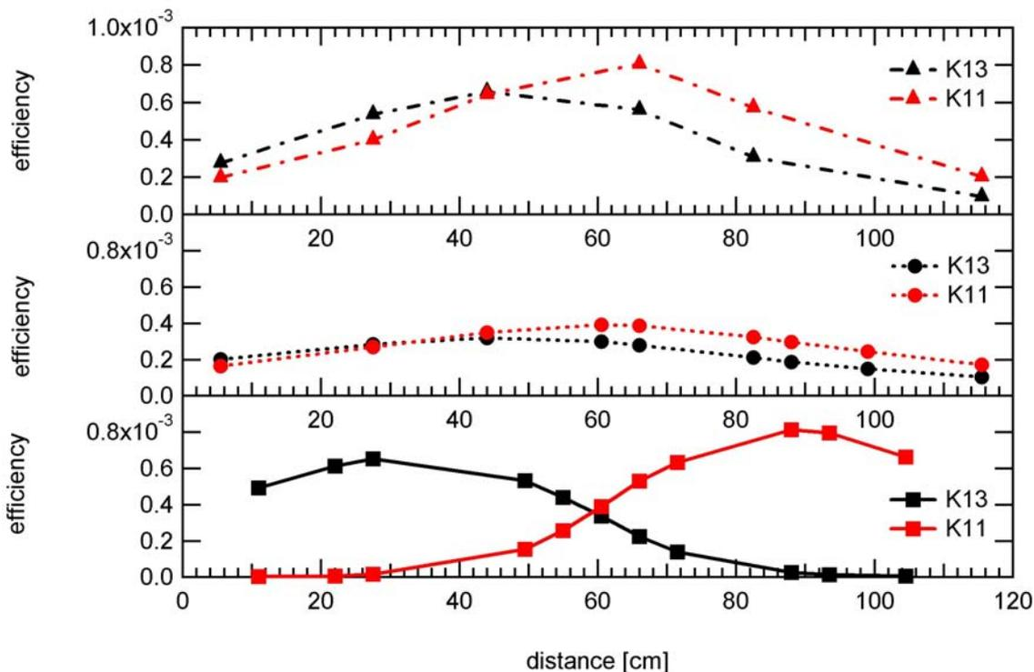
Figure 4.1. MCNPX simulation results for a polyethylene brick phantom. Each point has been calculated such a way that 30 cm long cylinder of  $^{60}\text{Co}$  was placed in different locations perpendicular to longitudinal axis of the phantom (Figure 2.2.). Top: Detectors were 15 cm apart and 26 cm away from the phantom. Middle: detectors 15 cm apart and 41 cm away. Bottom: detectors 37 cm apart and 26 cm away and there are lead collimators around each crystal narrowing the solid angle.
