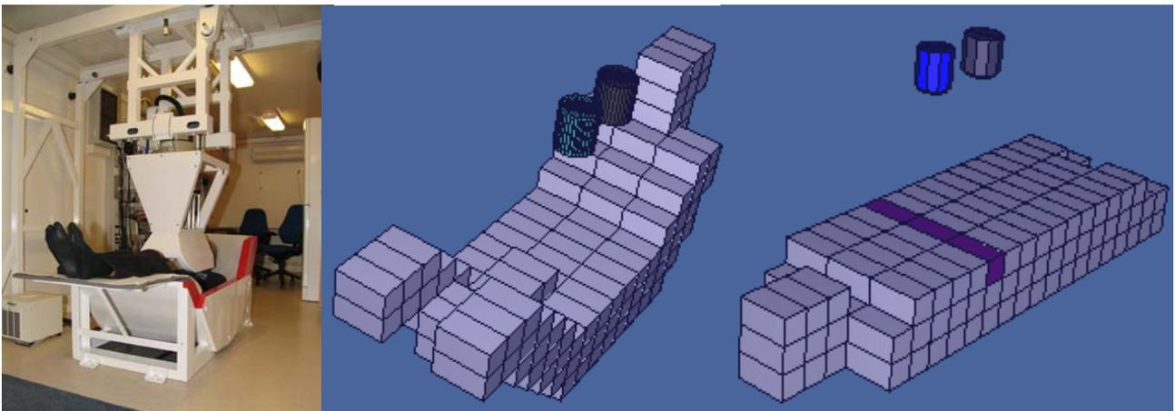
*Figure 2.2. Left: Inner view of the truck. Center: MCNPX model of the present setup. Right: New lie-down geometry. Lead made background shields are removed for clarity reasons.*
