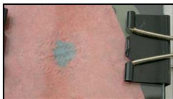
Fig. 1 A blue spot on the indication paper created after the sulfur mustard penetration through a sample of material
