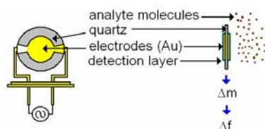
Fig. 2 QCM sensor working principle
