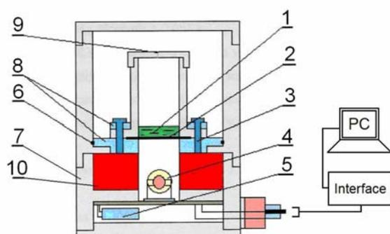
Fig. 3: A schema of the PIEZOTEST device permeation cell
