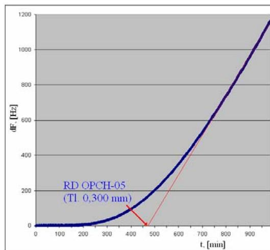
*Fig. 4 Graphical assessment of the insulating protective foil breakthrough time measured by the PIEZOTEST method*
